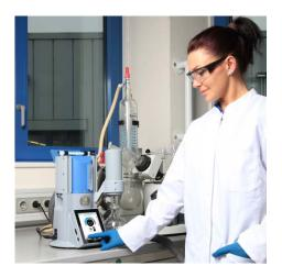
Automatic evaporation mode is perfect for controlling applications like rotary evaporation or vacuum distillation. Simply press the start button and the boiling pressure will be detected automatically and continuously adapted throughout the process. This makes the process run quickly, and without foaming. There's no need for manual adjustments or constant babysitting.
